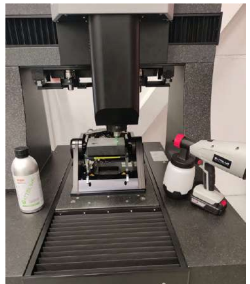
Coating Thickness Measurement with Alicona µCMM
